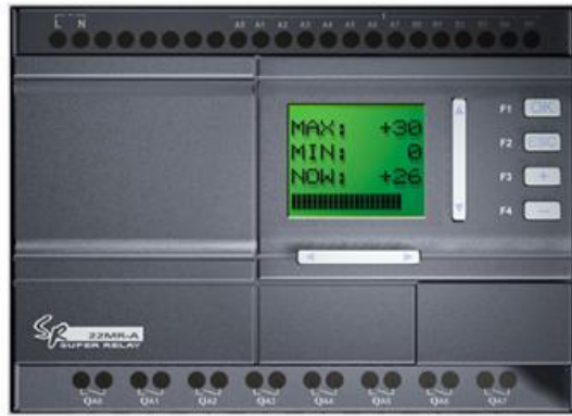
Fig. 3 SPR-22 Series PLC
